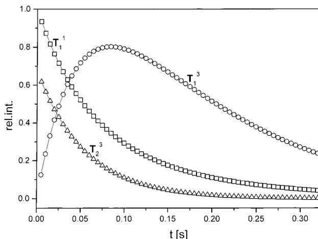
**Figure 3.** Time evolution of  ${}^7\text{Li}$   $T_1^1$  (rescaled 1/8),  $T_1^3$  and  $T_2^3$  in a 1 mol/L LiTFSI solution in a 1:1 w/w EODM-PC mixture.
