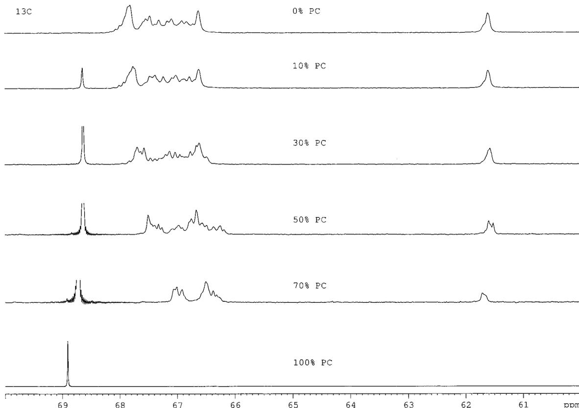
**Figure 7.** Relevant part of the  $^{13}\text{C}$  NMR spectra of the 1 mol/L LiTFSI solutions in the indicated (% w/w) EODM-PC mixtures.
