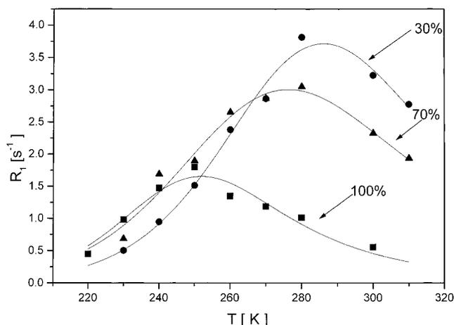
**Figure 1.** Temperature dependence of the  ${}^7\text{Li}$  longitudinal relaxation rate in a 1 mol/L LiTFSI solution in EODM-PC mixtures at the indicated PC concentration (% w/w).
