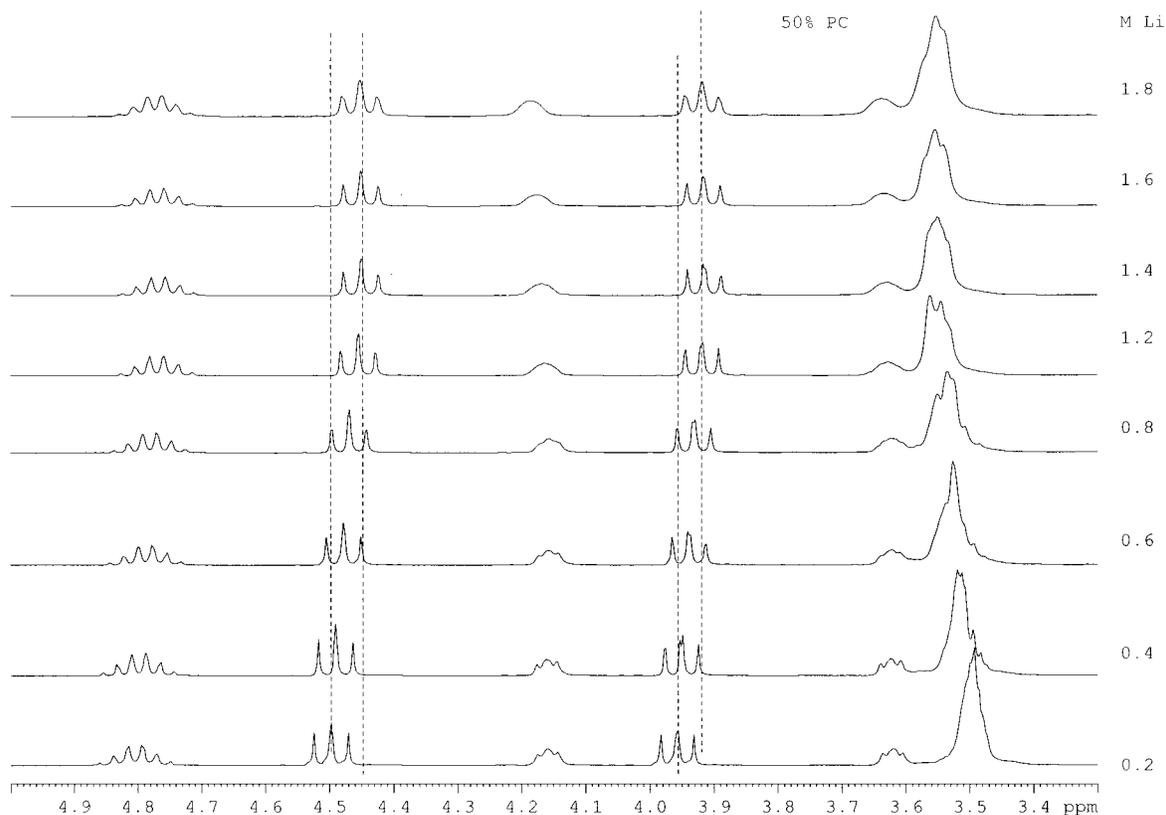
**Figure 4.** Relevant part of the  $^1\text{H}$  NMR spectra of LiTFSI solutions in a 1:1 w/w EODM–PC mixture at the indicated LiTFSI concentrations.
