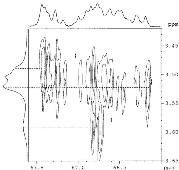
**Figure 8.** Relevant section of the  $^1\text{H}$ - $^{13}\text{C}$  HETCOR spectrum of the 1.2 mol/L LiTFSI solution in the 1:1 (w/w) EODM-PC mixture.
