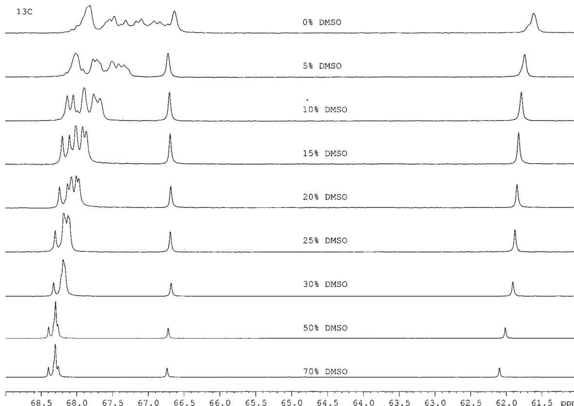
**Figure 14.** Relevant parts of the  $^{13}\text{C}$  NMR spectra of the 1 mol/L LiTFSI solutions in the indicated (% w/w) EODM–DMSO mixtures.
