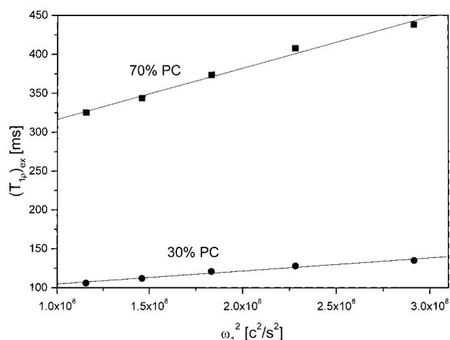
**Figure 2.** The linear dependence of  ${}^7\text{Li}$   $T_{1\rho}$  on the square of the spin-lock field intensity in a 1 mol/L LiTFSI solution in EODM-PC mixtures at the indicated PC concentration (% w/w).
