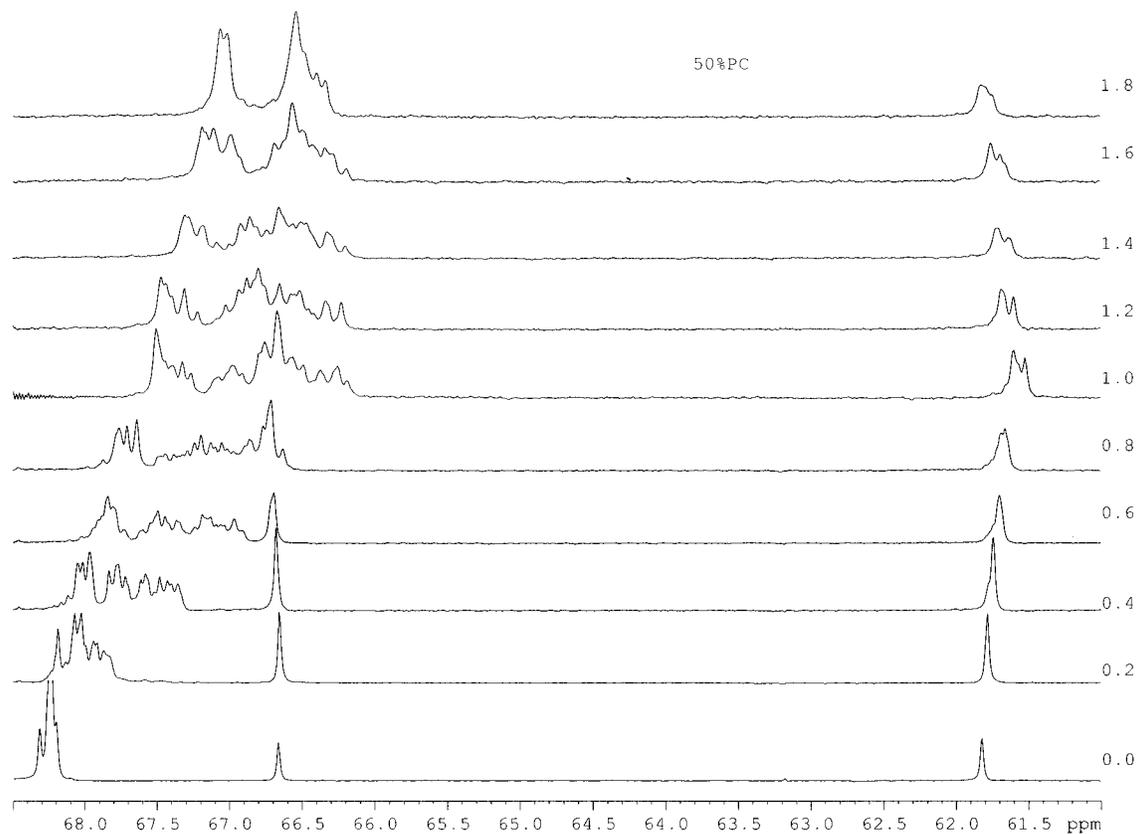
Figure 5. Relevant part of the  $^{13}\text{C}$  NMR spectra of LiTFSI solutions in a 1:1 w/w EODM-PC mixture at the indicated LiTFSI concentrations.
