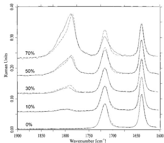
**Figure 10.** Relevant parts of the Raman spectra of the 1 mol/L LiTFSI solutions in the indicated (% w/w) EODM-PC mixtures compared with the (dashed) spectra of the same mixtures without LiTFSI.
