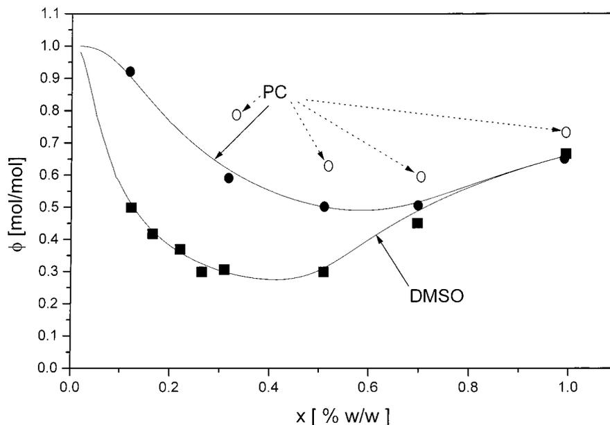
**Figure 15.** Fitted experimental values of the free solvent molar fractions obtained from  $^{13}\text{C}$   $T_1$  relaxation data of 1 mol/L solutions of LiTFSI in PC (●) and DMSO (■). The ○ points indicate the results obtained from Raman spectra.
