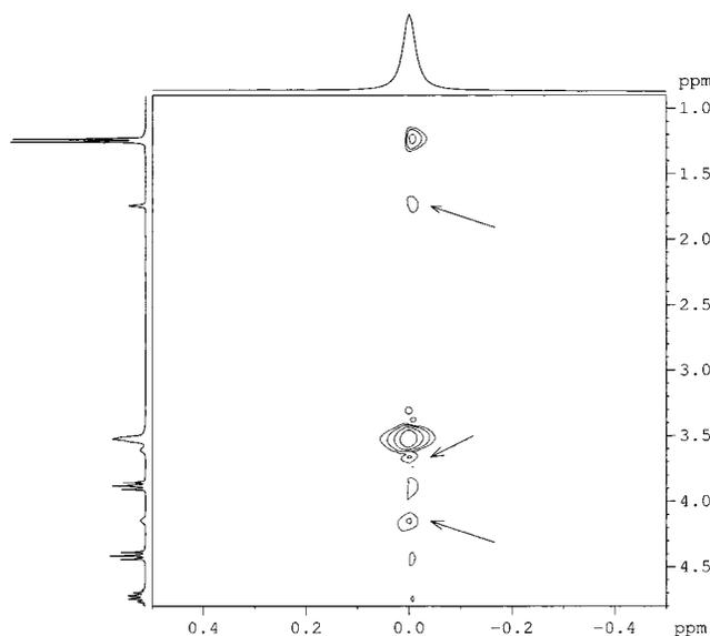
**Figure 9.** Relevant section of the  $^1\text{H}$ - $^7\text{Li}$  HOESY spectrum of the 1.0 mol/L LiTFSI solution in the 3:7 (w/w) EODM-PC mixture.
