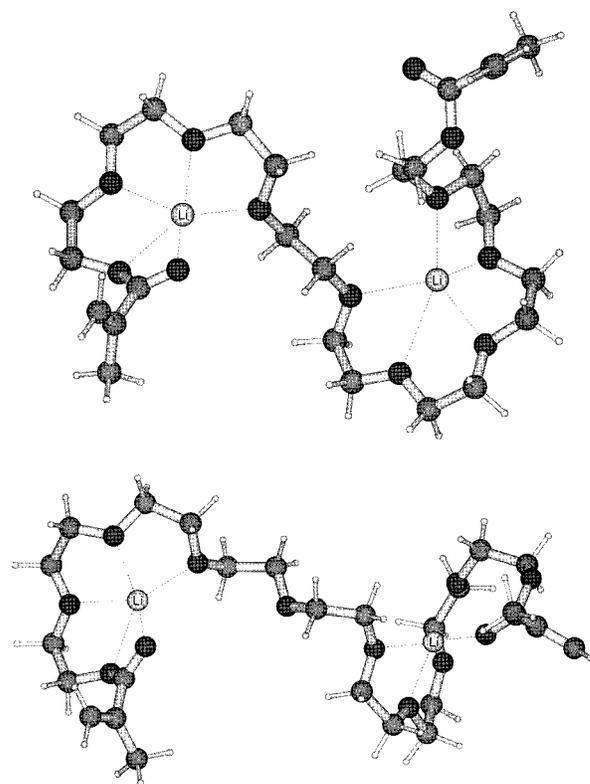
**Figure 11.** Two of the locally optimum geometries of the  $\text{Li}^+$ -EODM 1:1 and 2:1 coordinated structures according to MNDO.
