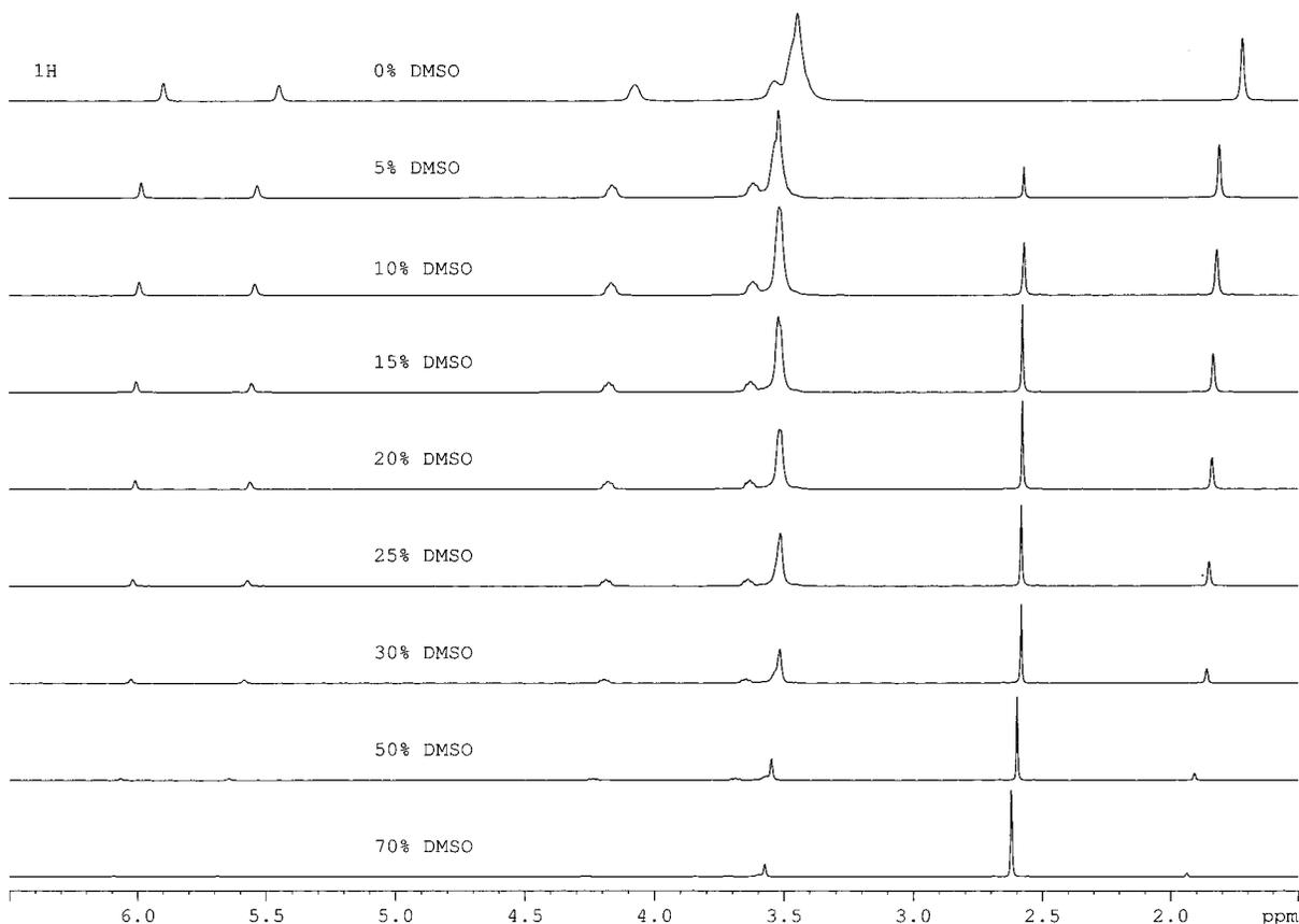
**Figure 13.** Relevant parts of the  $^1\text{H}$  NMR spectra of the 1 mol/L  $\text{LiTFSI}$  solutions in the indicated (% w/w) EODM-DMSO mixtures.
