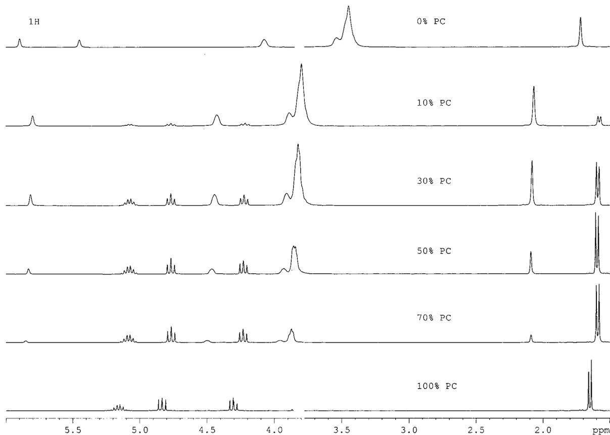
Figure 6. Relevant part of the  $^1\text{H}$  NMR spectra of the 1 mol/L LiTFSI solutions in the indicated (% w/w) EODM-PC mixtures.
